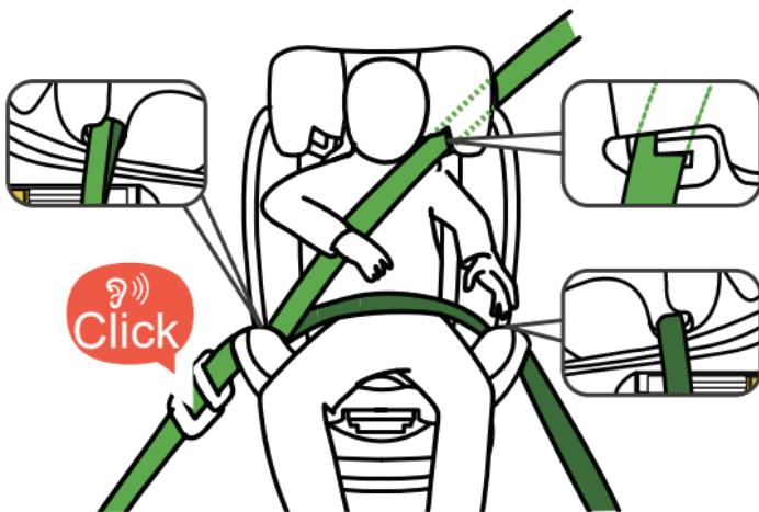
1. The 5-point seat belt and top-tether harness of the child car seat must be stowed as previously described. These are not needed in this size class.
