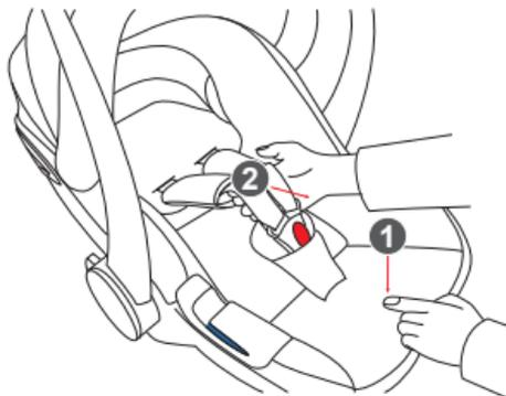
1. Loosen the shoulder straps by pressing on the central belt adjuster (1).
