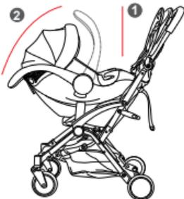
1. To attach the infant carrier, place the baby carrier on the adapters so they fit right and left into the bezel. The carrying handle must be in the foremost position (1). Press the baby seat down slightly so that the baby seat sits properly on the adapters.
