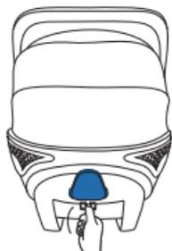
1. Release the lock on the flap by pressing the tab downwards.
