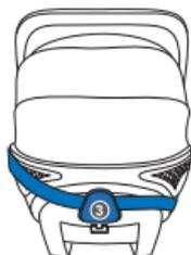
1. Pull the safety belt of the vehicle and carry out the lap belt under the side guide (1) right and left.
